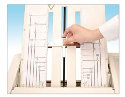
**FOLD PLATE GRAPHICS** Fold plates with clear graphics and measurements ensure accurate paper stop placement.
